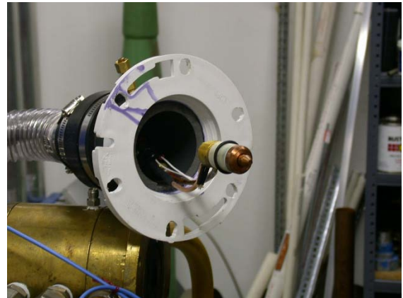
Fig. 11. Photograph of Hypertherm Plasma Torch showing modifications for methane operation.
